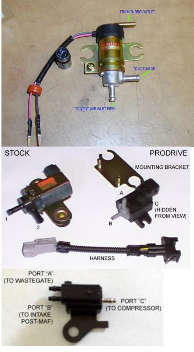
A = WASTEGATE B = INTAKE C = COMPRESSOR External Wastegate Plumbing
