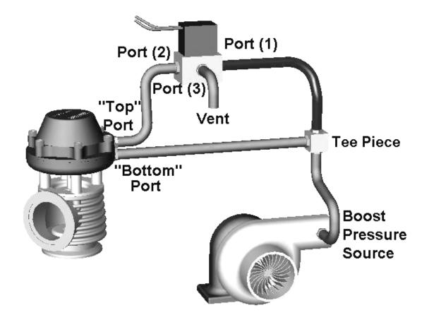
Above diagram is for Haltec/Turbosmart solenoid.
